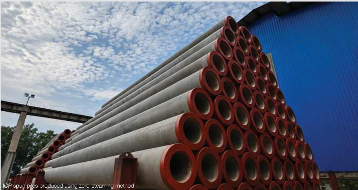
ICP spun piles produced using zero-steaming method
