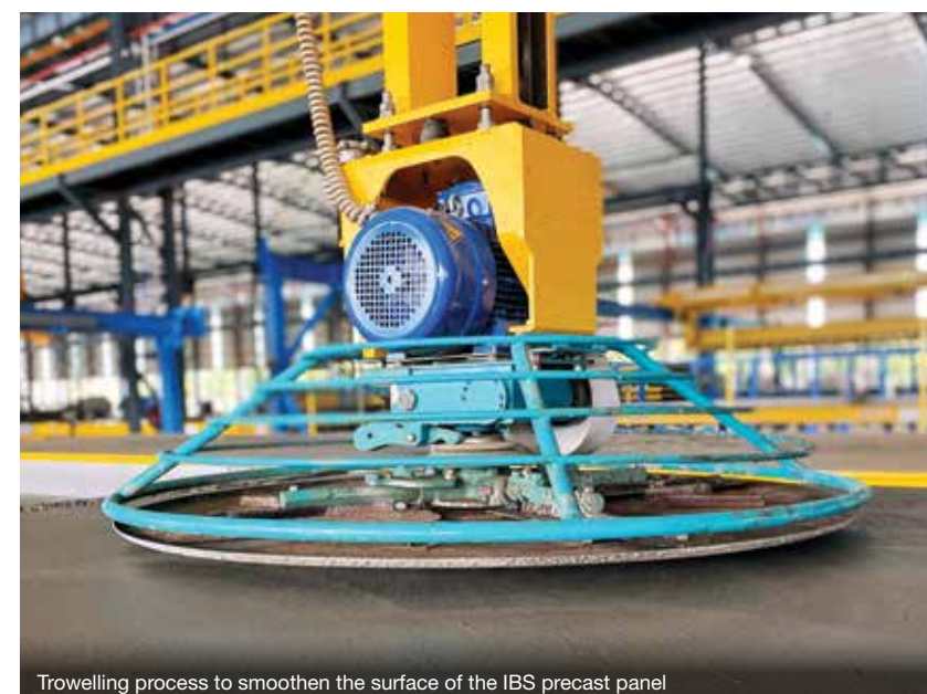
Trowelling process to smoothen the surface of the IBS precast panel
