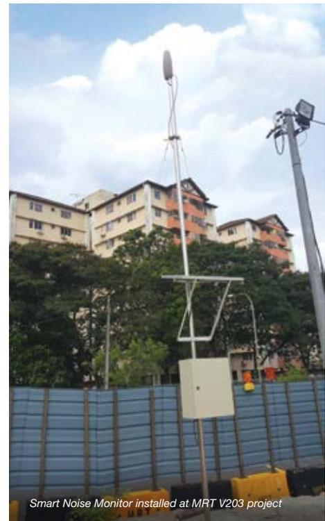
Smart Noise Monitor installed at MRT V203 project
