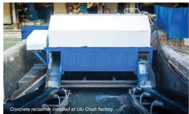
Concrete reclaimer installed at Ulu Choh factory
