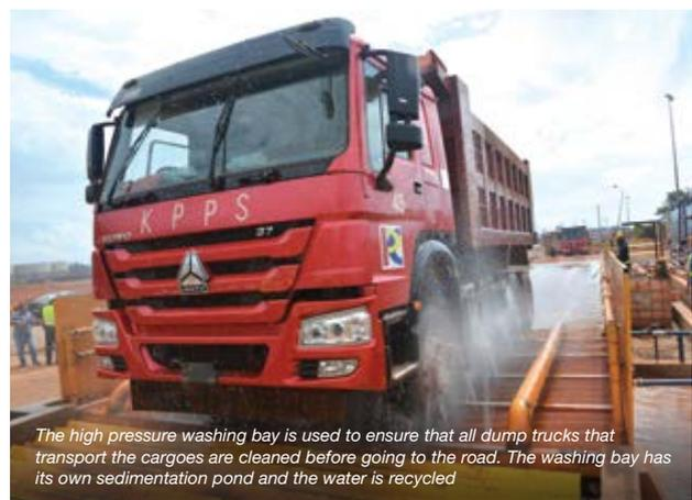
The high pressure washing bay is used to ensure that all dump trucks that transport the cargoes are cleaned before going to the road. The washing bay has its own sedimentation pond and the water is recycled
