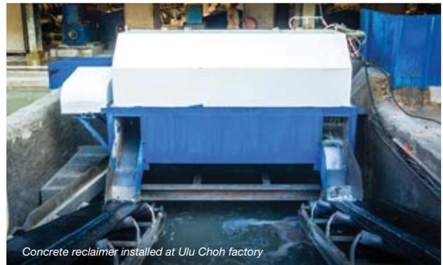
Concrete reclaimer installed at Ulu Choh factory
