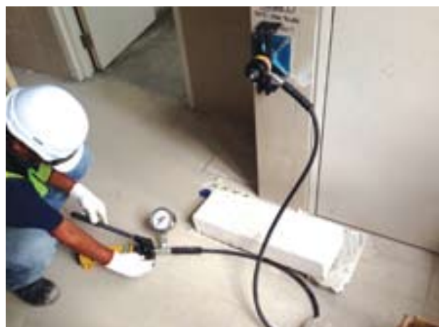
Pull Out Test on tiles is carried out to check and verify the strength of the adhesive achieved is in accordance with the requirements
