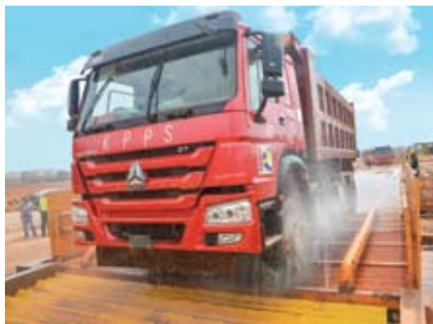
Wheel washing facility to minimise dust pollution
