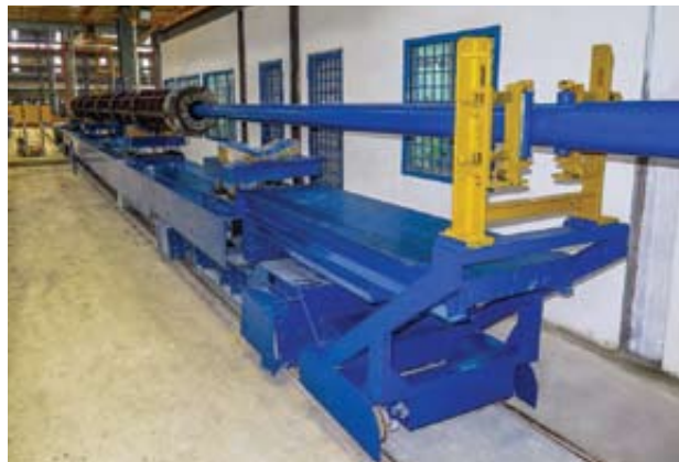
Process improvement for concrete pumping system to prevent the pipe from wobbling and touching the mould, thus preventing errors of inaccurate concrete weight
