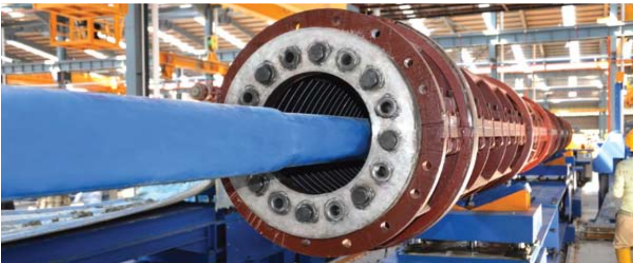
Concrete feeding process of ICP Piles using concrete pumping technology
