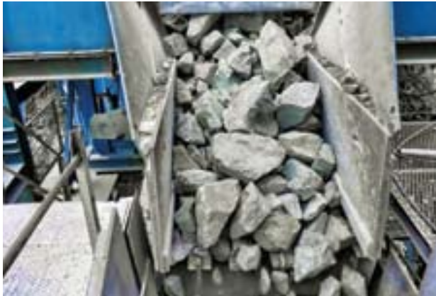
Blasted rock from primary hopper to jaw crusher at Kuantan Quarry
