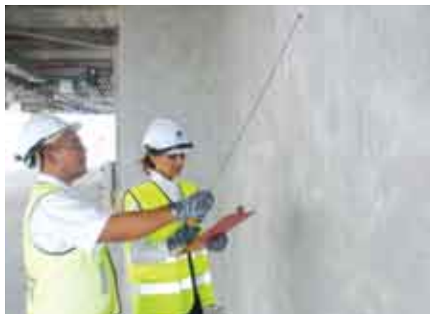
Quality assessment at Platinum Park Phase 3 project: A metal tapping rod is used to detect the hollowness of the plaster finish surface
