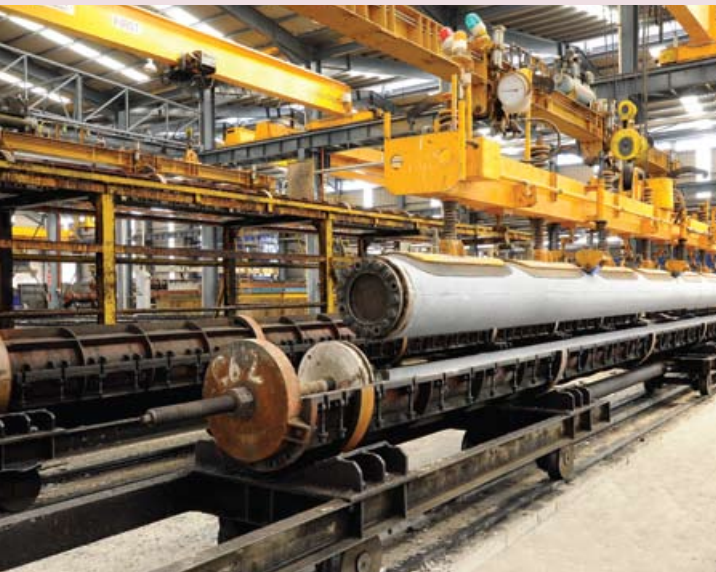
Pile being lifted with a vacuum lift during demoulding process
