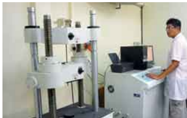
Industry Division's Research & Development Centre: Testing for durability and strength of PC bars
