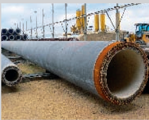
Biggest pile developed with diameter of 1400mm by ICP Jiangmen, China
