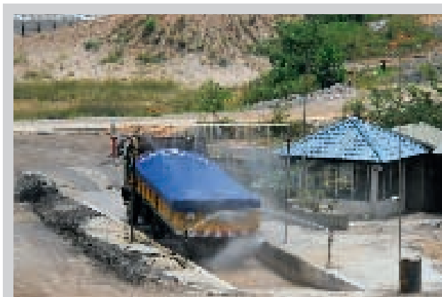
Sprinkler system used to dampen down the load on the lorries at our quarries
