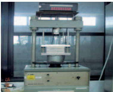
Resilient modulus test equipment used to test cored premix at our projects
