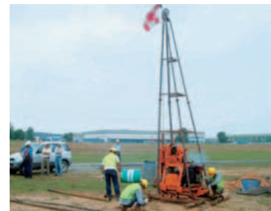
Deep soil boring test is performed at project site
