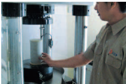
Compression test for concrete cylinder for a USA project at an independent laboratory
