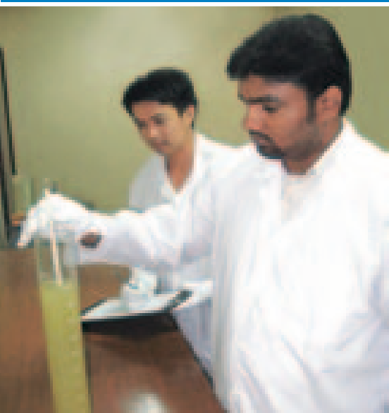
Specific gravity test in Industries Division's R&D laboratory to determine volume of PCE Admixture in Grade 80 PSC piles
