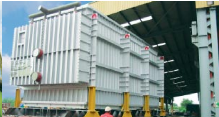
80 ton Waste Heat Recovery Unit for Shell LNG Plant in Nigeria
