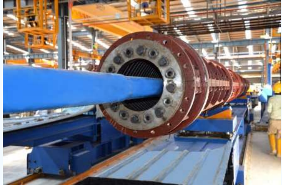
Concrete feeding process of ICP Piles using concrete pumping technology
