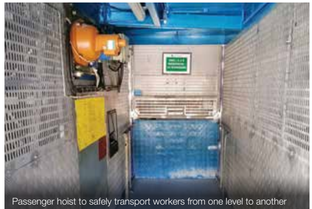
Passenger hoist to safely transport workers from one level to another
