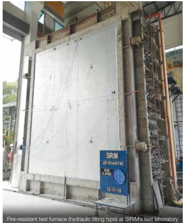
Fire-resistant test furnace (hydraulic tilting type) at SIRIM's test laboratory
