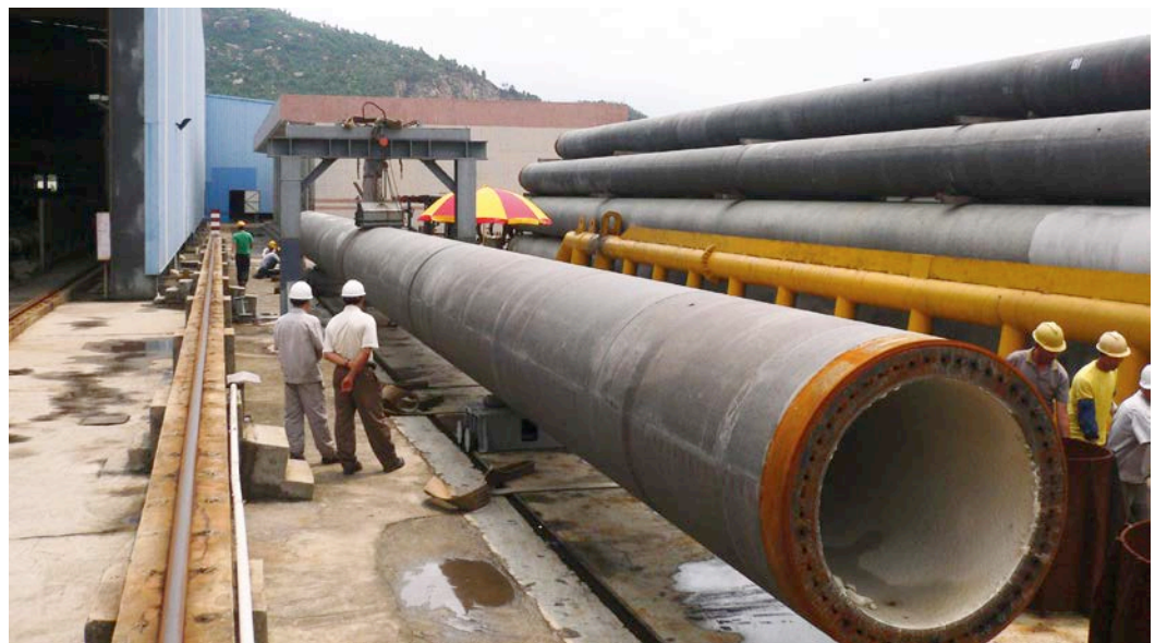
The largest pile with a diameter of 1,400mm manufactured by ICP in Jiangmen, China.
