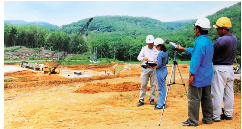
IJM adhered strictly to the Putrajaya local authority's noise pollution levels. Picture here shows project staff measuring noise generated by construction machinery near a residential area in Jalan Lingkaran, Putrajaya.
