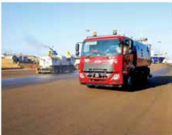
The road sweeper and road water jetter during a routine road cleaning activity at the Port
