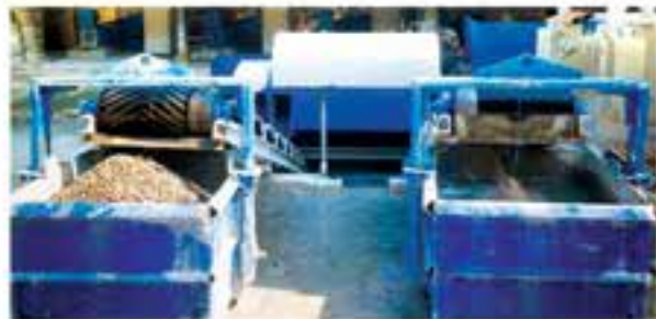
The recovered aggregates and sand are mixed into the stockpile and reused in production
